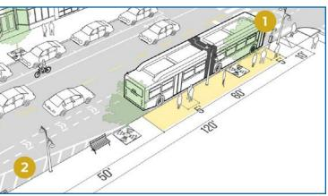
• Locate stop zone with at least 10 feet of clear distance from crosswalk or curb return. Measure to transit stop pole at near-side, or rear of transit vehicle at far-side.
