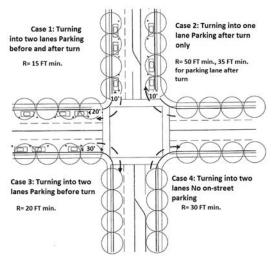
Intersection Design for Bus Turns (source: Tri-Met)
