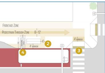
For pedestrian access to stops, a minimum four-foot-wide clear pedestrian travel path should be provided to connect the bus stop waiting area and loading area to adjacent development or neighborhoods, though eight-12 feet is preferred where transit is present; the pedestrian travel path may be wider based on pedestrian and transit rider capacity (NACTO, 2016). The travel path should have a non-slip surface to meet ADA
